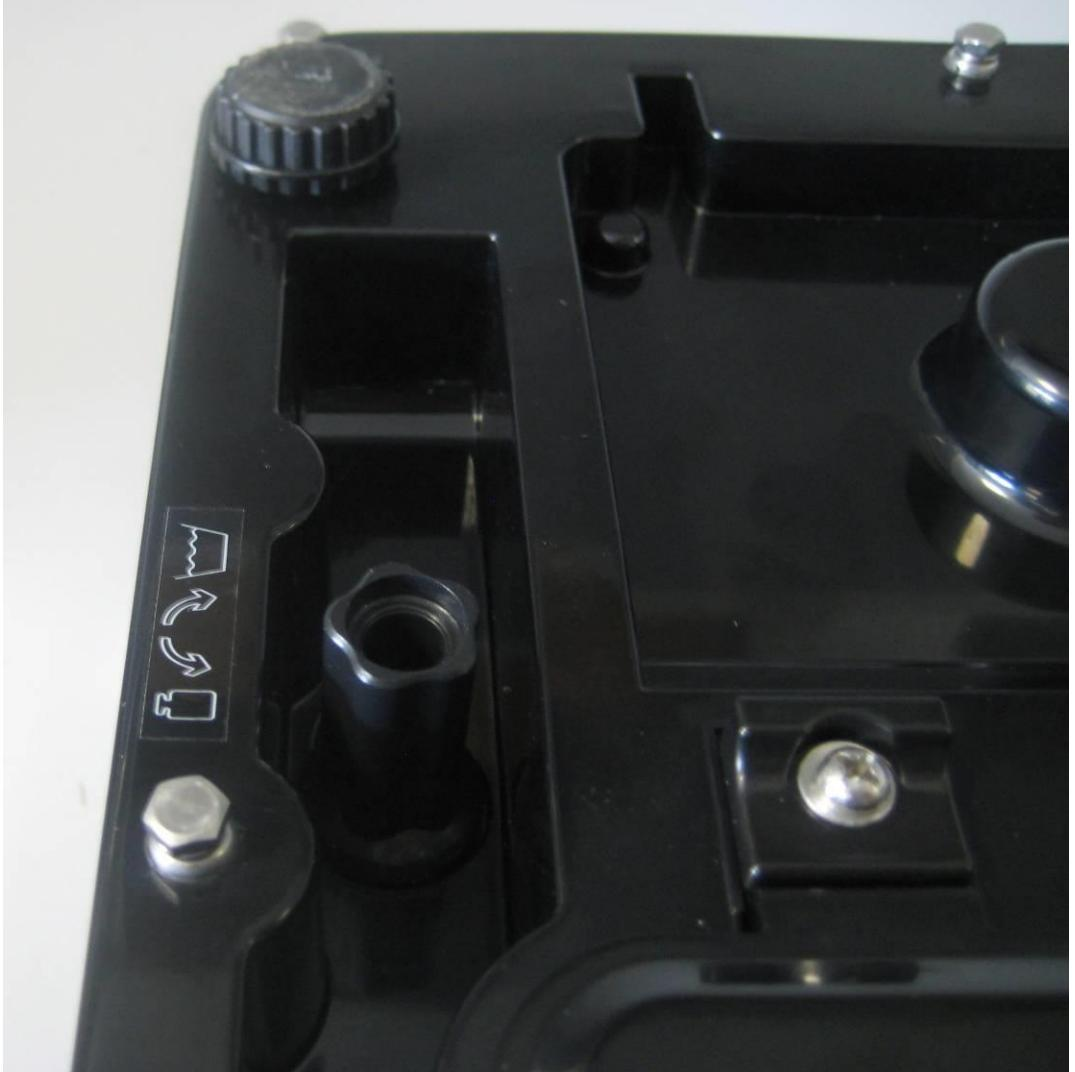
c) Level the platform by adjusting the adjustable feet. The stability of the platform is very important.
